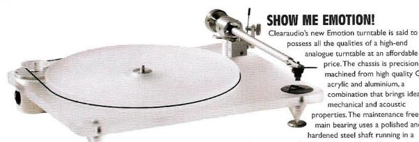
properties. The maintenance free main bearing uses a polished and hardened steel shaft running in a polished sintered bronze precision cap. The motor is isolated and damped from the chassis, driving the precision-machined 20mm thick turntable platter via a polished jointless drive belt. Speed selection of 33 1/3 and 45 rpm is easily achieved by changing the position of the drive belt
