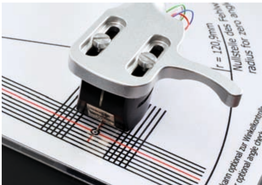
The best adjusting gauge? Comes with the individual tone arm. Clearaudio describe in detail how to fine-tune the pickup.
