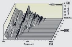
ABOVE: Cumulative tonearm resonant decay spectrum, illustrating various bearing, pillar and 'tube' vibration modes spanning 100Hz-10kHz over 40msec
