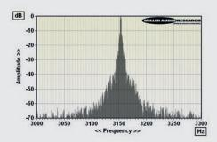
ABOVE: Wow and flutter re. 3150Hz tone at 5cm/sec (plotted ±150Hz, 5Hz per minor division). Absolute speed accuracy can be finely adjusted by the user
