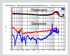
The frequency response takes a very straight path in the bass and mid-range area. At the very top there is the slight rise typical of MCs. However, at around 5dB at 20KHz, it is very modest. With a platter rumble is at 73dB and with a coupler at 83, while the fluctuations in even speed of ±0.068% are also excellent.
