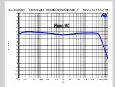
With S/N ratios of 78 dB (RCA input) and greater 80 dB (XLR) the Absolute Phono has very good noise values. The frequency response shows a limitation at around 40 kHz and a very little bass and treble boost of about 0.5 dB each. The low-Z (64  $\Omega$ ) XLR output can also drive longer cables easily.
