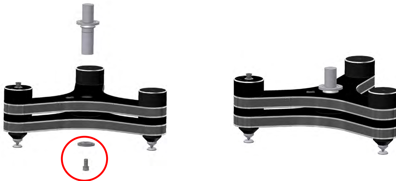
Pic. 8: Setup of the drive bearing
