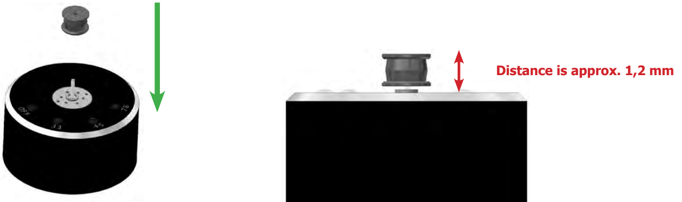
Pic. 10: Setup of the Master Innovation pulley
