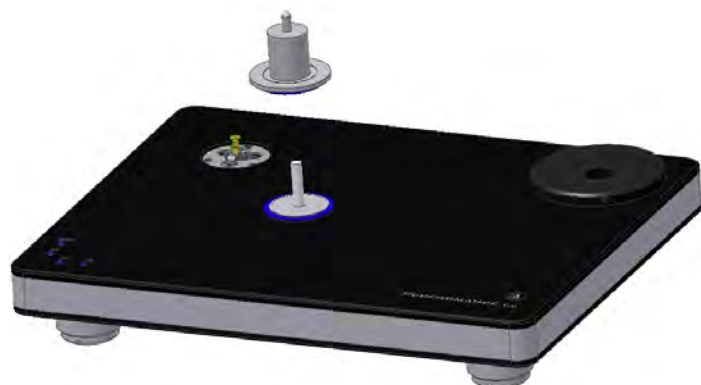
Pic. 6: Fitting the bearing upper part
