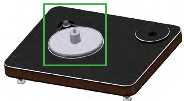
Pic. 7.1: Placing the belt
