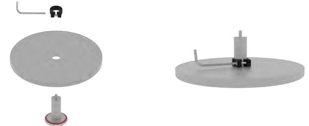
Pic. 9: Connection of sub-platter and bearing
