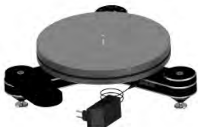
Pic. 11: Connection of power supply and motor
