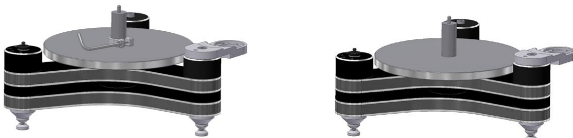
III. 7: Retirer le collier de serrage
