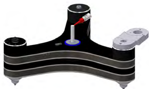
Pic. 6: Oiling the bearing shaft
