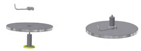
Pic. 7: Connection sub-platter and bearing upper part
