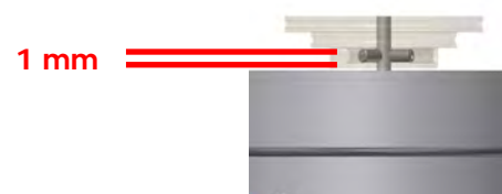
Pic. 12: Mounting the pulley
