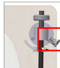
Illustration 3 : Maximum antiskating (Screw is screwed in)
