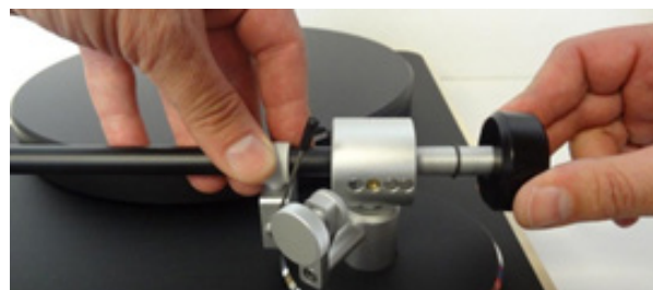
Pic. 2: Installing the counter weight
