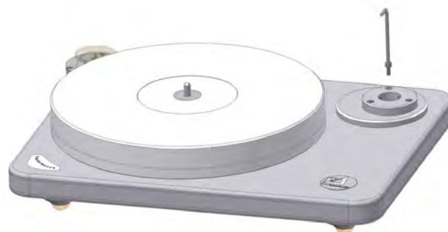
Pic. 3: Mounting the tonearm base
