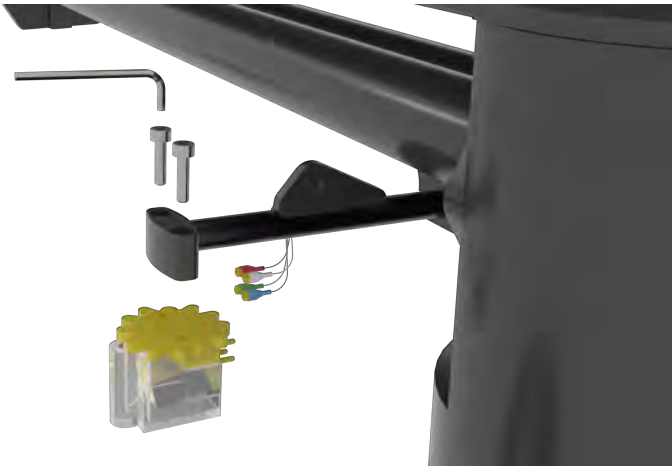
Pic. 14: Mounting the cartridge
