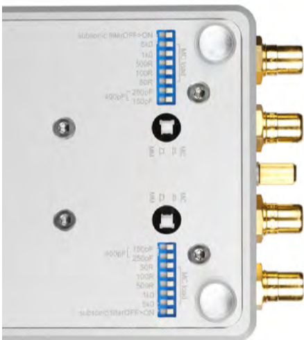
Pic. 3.1: View from the bottom side
