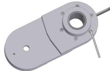
**Pic. 3:** Tighten the *VTA-Lifter* in a Solution base
