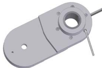
Pic. 3: Tighten the VTA-Lifter in a Solution base
