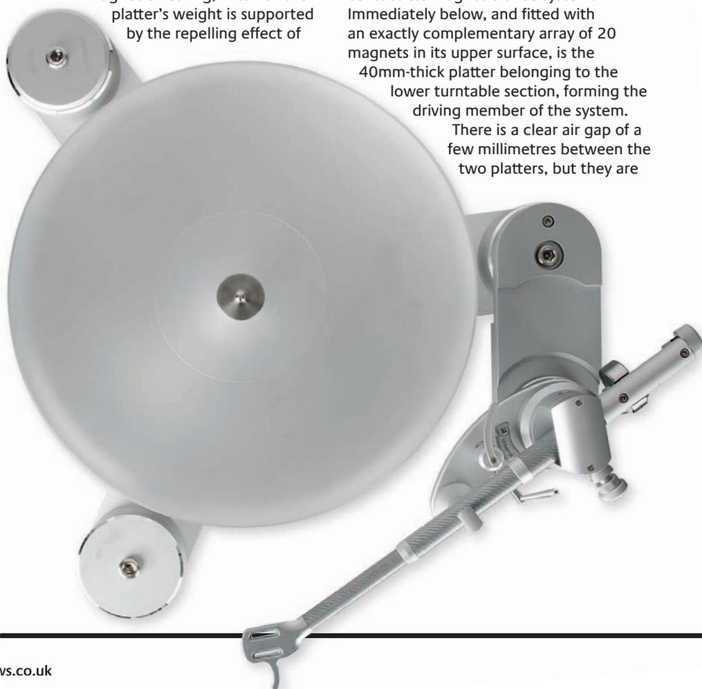
**RIGHT:** Running on Clearaudio's patented Ceramic Magnetic Bearing magnetic bearing is a 70mm-thick acrylic main platter. The version that comes in a black finish has a softer POM platter, which may give a slightly different sound
