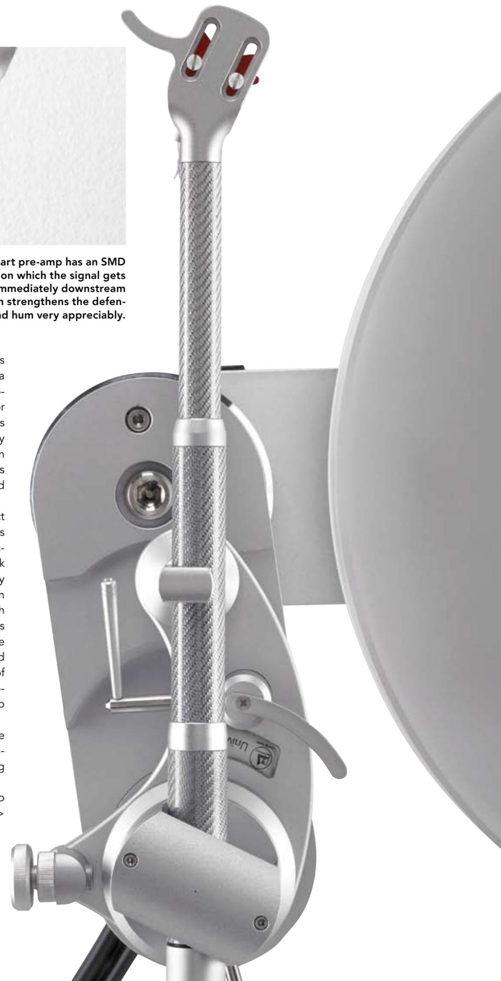
Right on the wire: eight solid core silver leads - two each per channel for symmetric signal transfer and power - connect the outpost, placed right at the front, with its base station.
