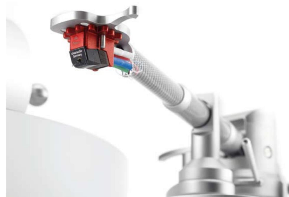
**Da Vinci Red: within its aluminium casing covered in a red ceramic coating the moving coil system houses lightweight, fine gold coils, plus eight magnets for a high degree of effectiveness and perfect symmetry.**
