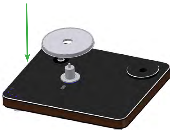
Pic. 7: Setting the sub-platter
