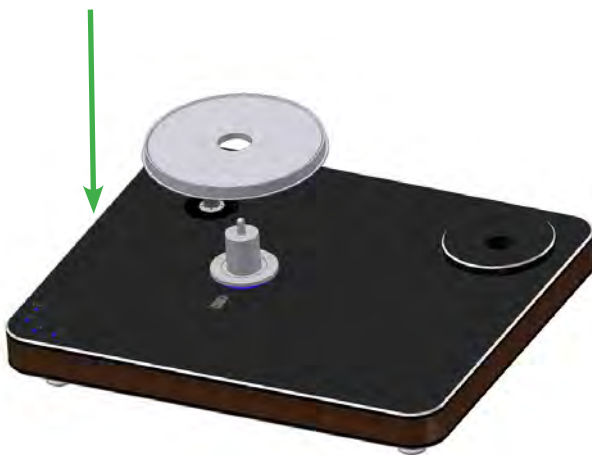
Pic. 7: Setting the sub-platter
