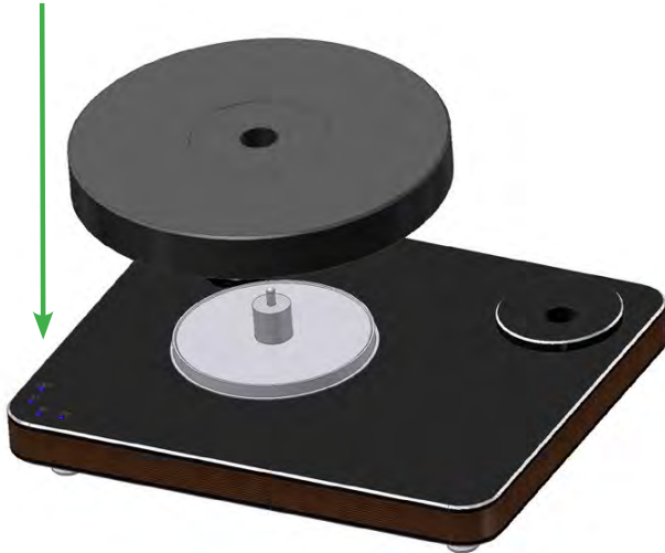
Pic. 8: Setting the platter onto the bearing
