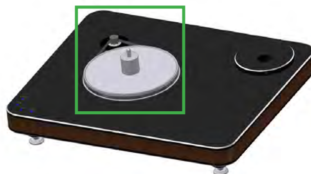
Pic. 7.1: Placing the belt
