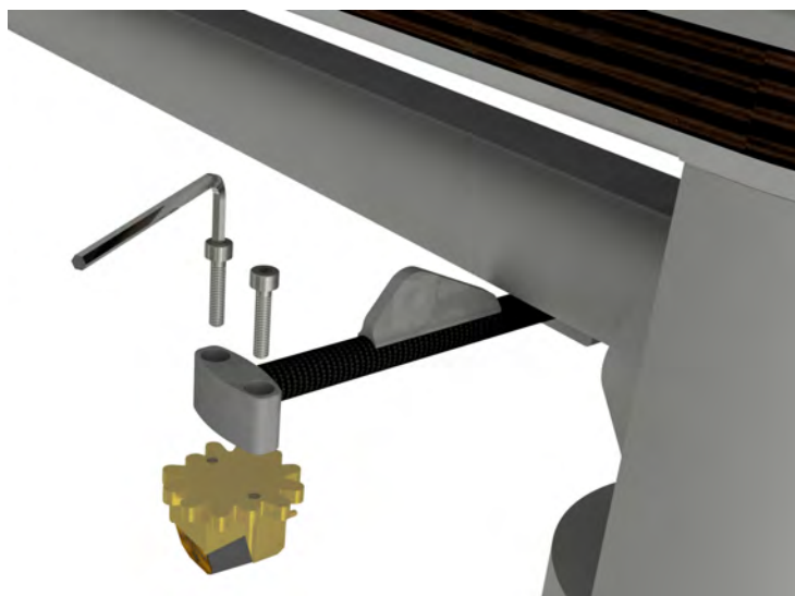
Pic. 15: Mounting of the cartridge
