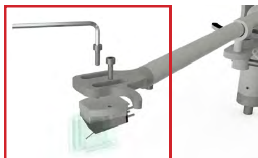
III. 6: Installation de la cellule
